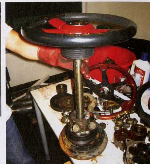
廢棄的剎車碟已經磨損，但非常適合作為椅子或桌子的底座 Discarded brake disc was chosen for its weight and shape as the base of a stool or coffee table
