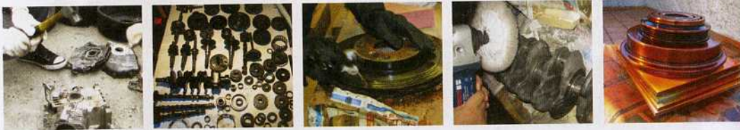
收集回來的零件需先作處理，這包括解體、分類、清潔、打磨及拋光上油（從左至右） Collected car parts must be taken apart, classified, cleaned, polished, burnished and painted before use
